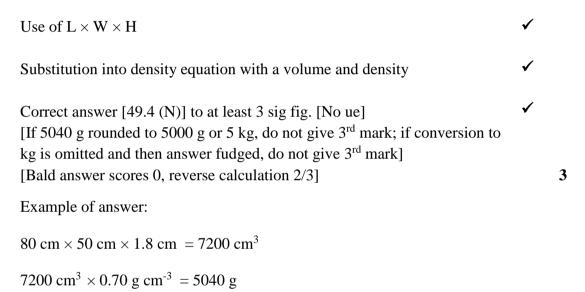
$5040 \times 10^{-3} \text{ kg} \times 9.81 \text{ N/kg}$
